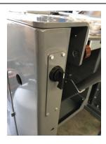
To center the Mover with the work plate turn the rotary airswitch.
